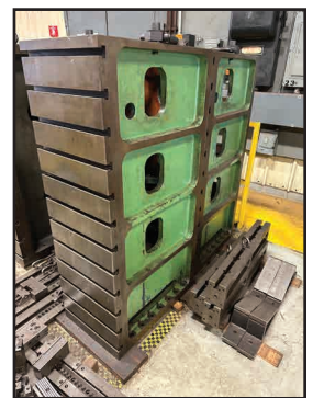
VIEW OF BOX TABLES
